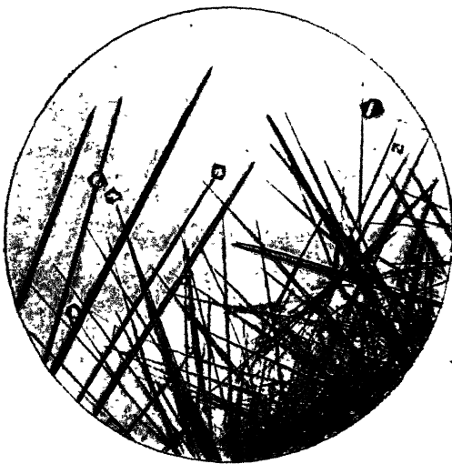
FIG. 55.—Rhombic Needles and Cubic Octahedra of Antimony Trioxide obtained by Sublimation. An interesting Example of Dimorphism
